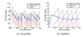
Fig. 11. Instability and stability of the ALT algorithm. In (a), a=100, b=1, the maximum buffer size is 50000 packets. In (b), a=10, b=1, the maximum buffer size is 400 packets. In both figures, there is 1 download and no upload.
